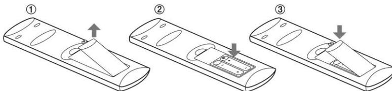
Open the battery door and insert the batteries.
