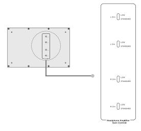
Headphone Amplifier Gain Control switch: the default setting is "Standard" mode. When you use IEMs, please set it to "Low" mode. Make sure the four switches are at the same mode setting.
