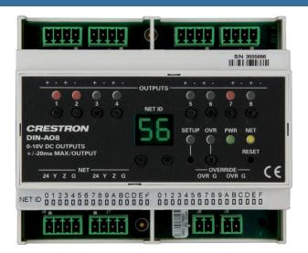
**OVERRIDE:** (2) 2-pin 3.5mm detachable terminal blocks, paralleled; Sensing input for external low-voltage contact closure; Activates override mode when a closure is present; Minimum Closure Rating: 10mA (per module) at 24 Volts
